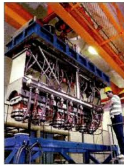
A cryostat from the injector of Argonne's ATLAS. It contains six, four-gap, quarter-wave resonators. The RIA linacs use superconducting technology over the ion velocity range of 2–85% of the speed of light. The development of superconducting resonators for RIA is in progress at Argonne, Michigan State and Jefferson Lab.
