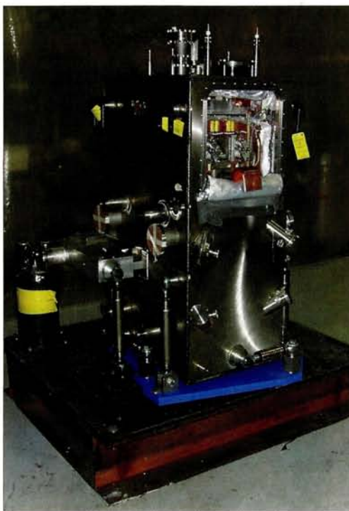
A superbend magnet in its cryostat awaiting characterization measurements.
